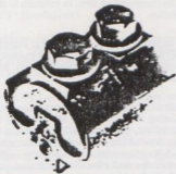
FIG. 4 - Aluminium to Aluminium Connector
