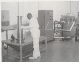
FIG. 8: Epoxy Resin Casting Plant
