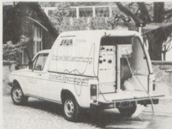
Typical vehicle mounting arrangement of BAUR Syscompact cable fault location and test equipment.
