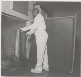
FIG. 14: Mould With Casting In Second Stage Cure Oven
