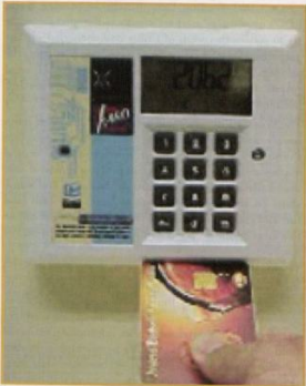
Figure 3 - A Smartcard Prepayment Multi-Utility Meter Interface
