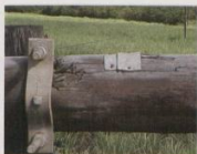
Fig. 4: The initial tracking on wood surface in areas where pollution plays a role can be seen in Fig. 4(a). The ignition of the wood and destruction of the structure can be seen in Fig. 4(b). The leakage current is a function of the pollution in the area, the type of insulators used on the structure and the number of parallel leakage paths that are available on the structure.
