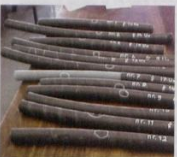
Fig. 6: Breakdown sites of the twelve 500 Hz aged MV XLPE cable core samples.
