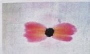
Fig. 1: Bowtie water tree growing from dust particle in six-year old XLPE insulation.
