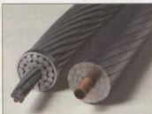
Fig. 2: Conventional ACSR and modern ACCC conductor.
