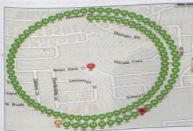
Fig. 6(a): Data concentrator indicating one faulty meter.
