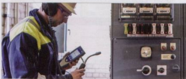
Fig. 9: EA Technologies UltraTEV Plus handheld PD tester unit.
