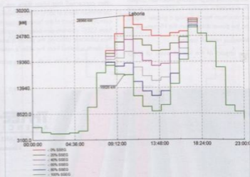
Fig. 10: Power flow with peak winter loading and varied levels of SSEG penetration.
