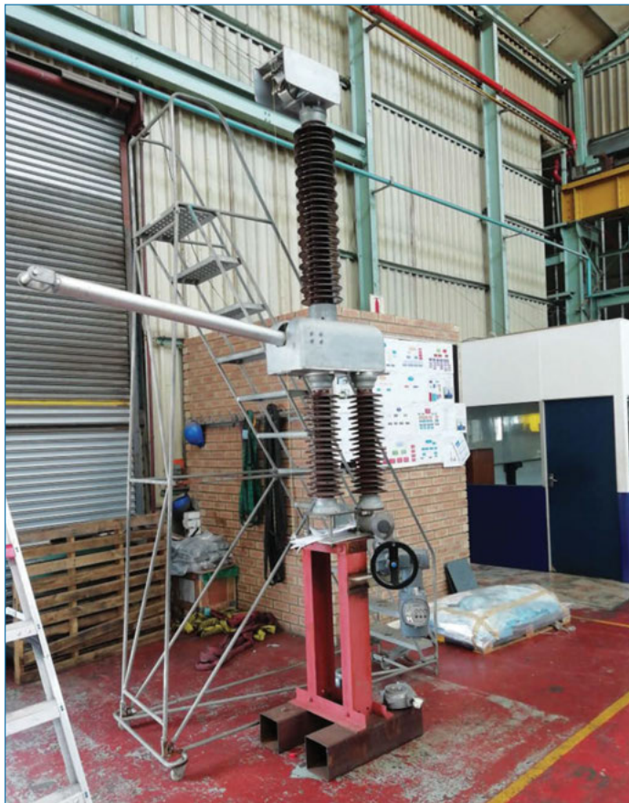
One of the special VM 132kV isolators in the ACTOM factory.
