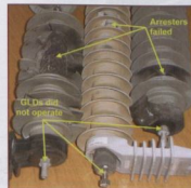
Fig. 3: The GLDs did not operate when the arresters failed.
