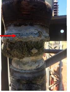
Location of erosion and electro-thermal failure
