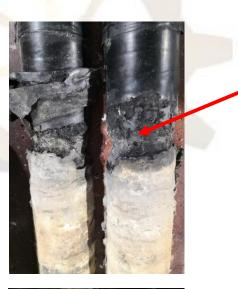
Erosion & Thermal Failure
