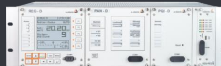
Voltage Regulation REG-D + Monitoring + SCADA
