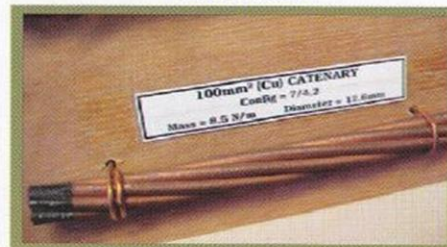
Catenary Wire 100mm 2 : Unit made from copper
