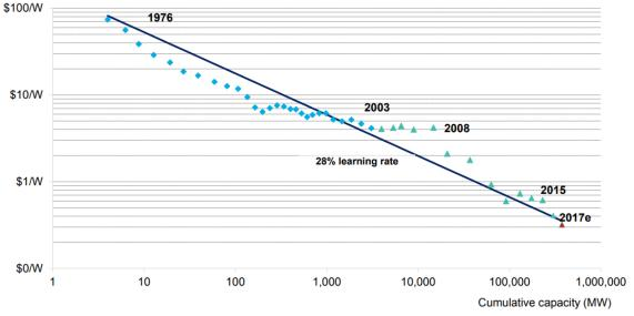
Figure 1: Crystalline silicon solar PV experience curve [1]
