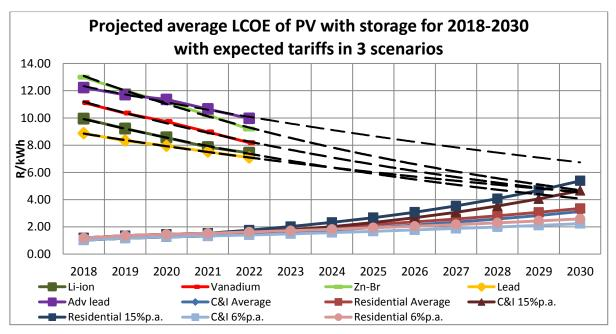
Figure 11: Average forecasted LCOE of PV with different technologies of storage for 2018-2030 plotted with Eskom electricity tariffs in 3 scenarios
