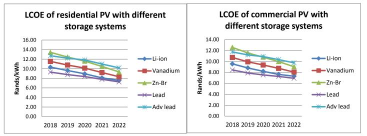
Figure 10: Average LCOE reduction for residential PV systems with different storage technologies for years 2018-2022
