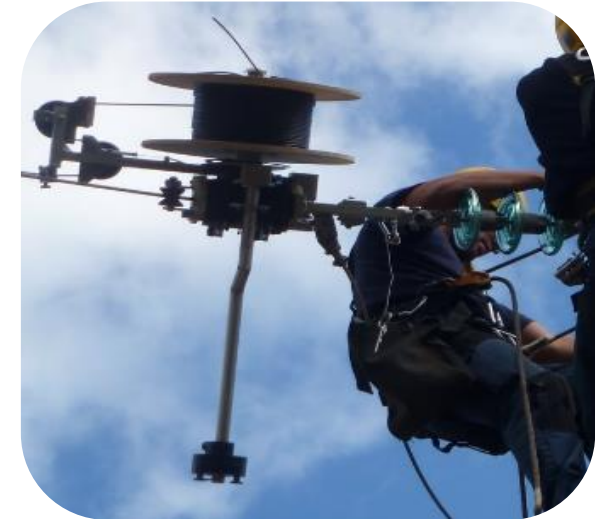
Local distribution lines (6-25kV) All-Up-Weight = 43kg
