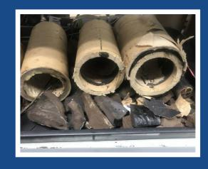
FR PVC cable samples after the TerraLoc and cardboard tubes were removed. Casting marks were present on the sheaths, but no cracks. The sheaths were still intact.
