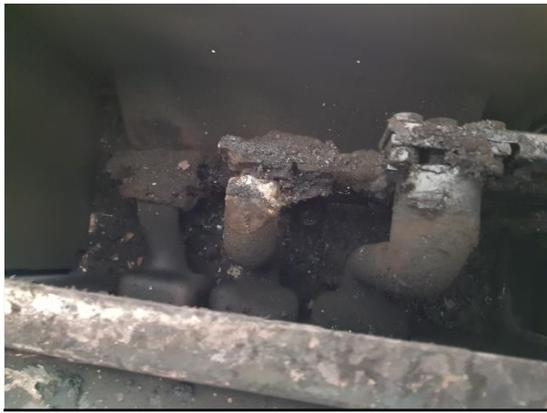
Fig. 13: 11 kV Busbar failure
