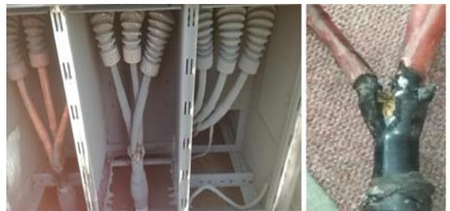
Fig. 12: 11 kV switchgear cable termination failure
