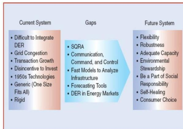
Figure 8: The transition from the current grid to the future grid (SQRA: Security, Quality, Reliability and Availability; DER: Distributed Energy Resources) [8]
