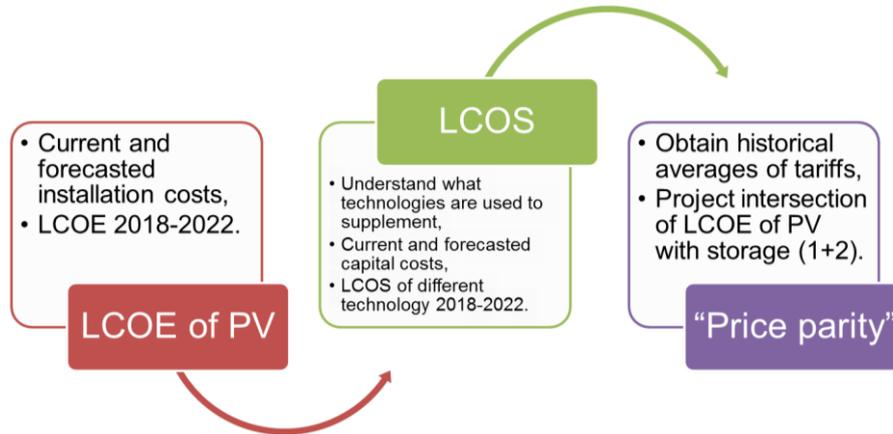
**Figure 3: Methodology used to determine LCOE of PV with storage**
