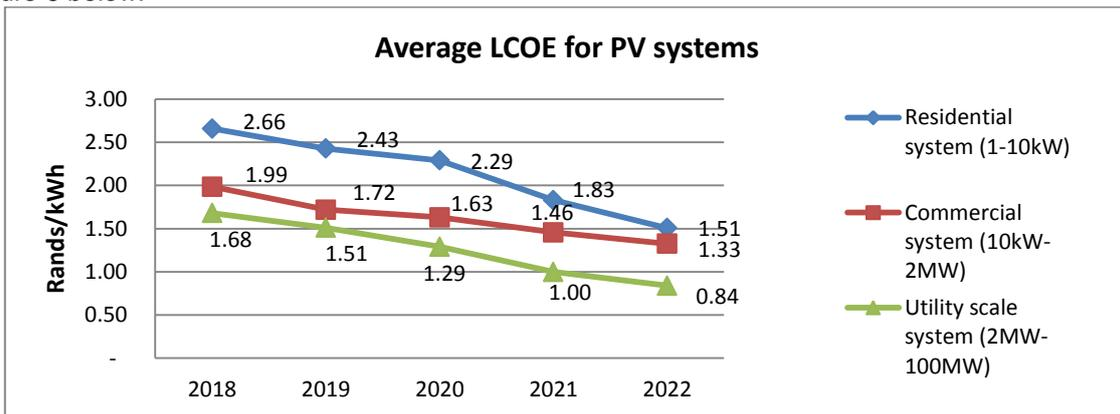
**Figure 6: Average LCOE (R/kWh) of PV systems from 2018-2022**
