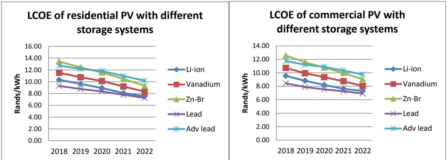
Figure 10: Average LCOE reduction for residential PV systems with different storage technologies for years 2018-2022
