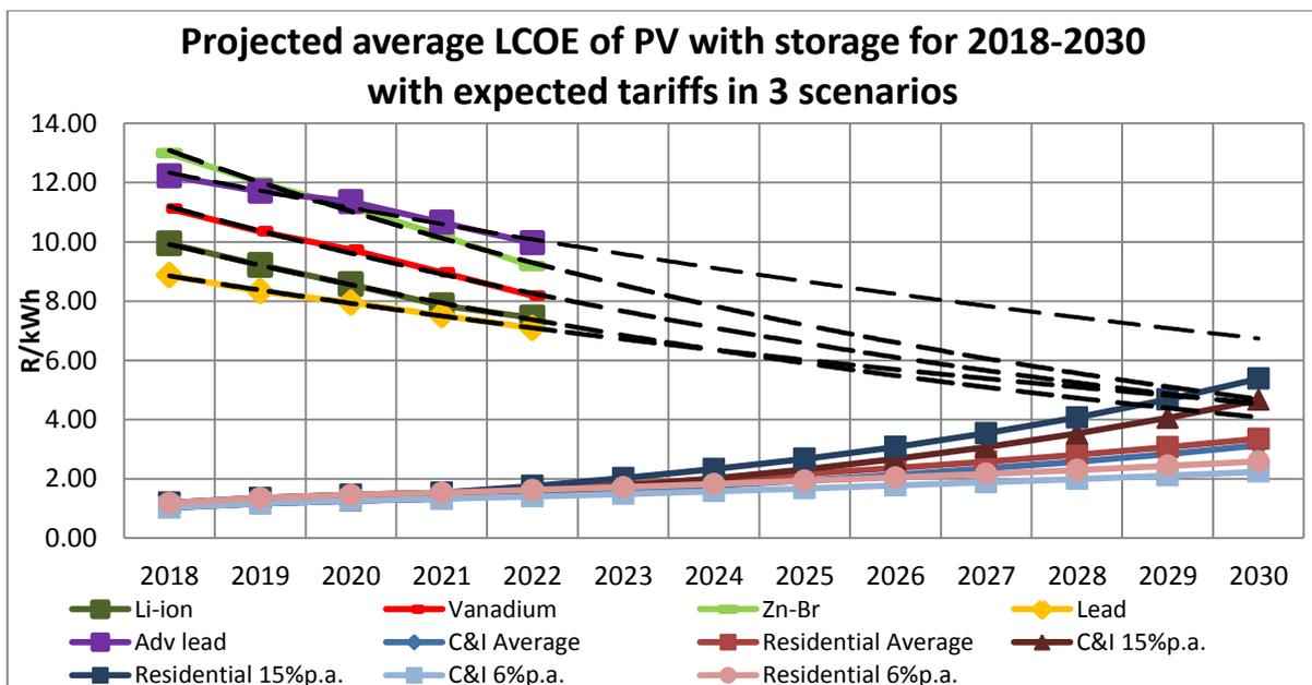
Figure 11: Average forecasted LCOE of PV with different technologies of storage for 2018-2030 plotted with Eskom electricity tariffs in 3 scenarios
