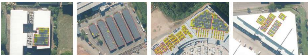
Figure 4: Errors of omission in the New Zealand model are particularly prevalent in large solar arrays
