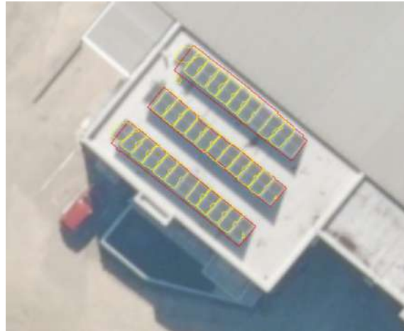
Figure 2: The USA model (red areas) identifies the entire solar panel array as a single feature, while the New Zealand model (yellow areas) differentiates according to individual panels.
